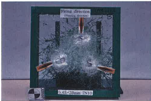
Figure 1 : Strike face of 12MB03373 after experiment
